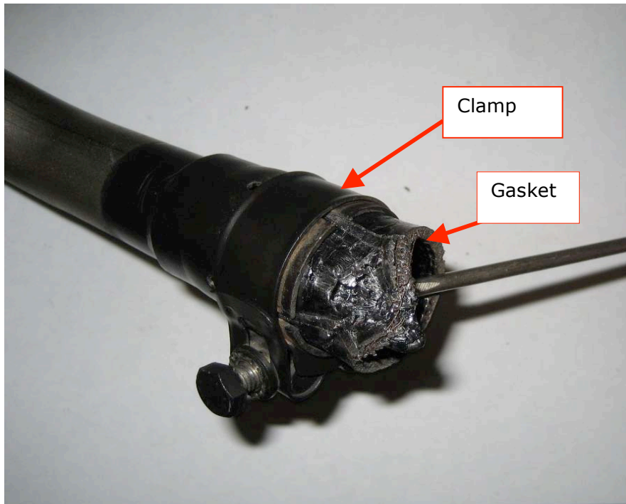
Remove the exhaust packing and clamp.
